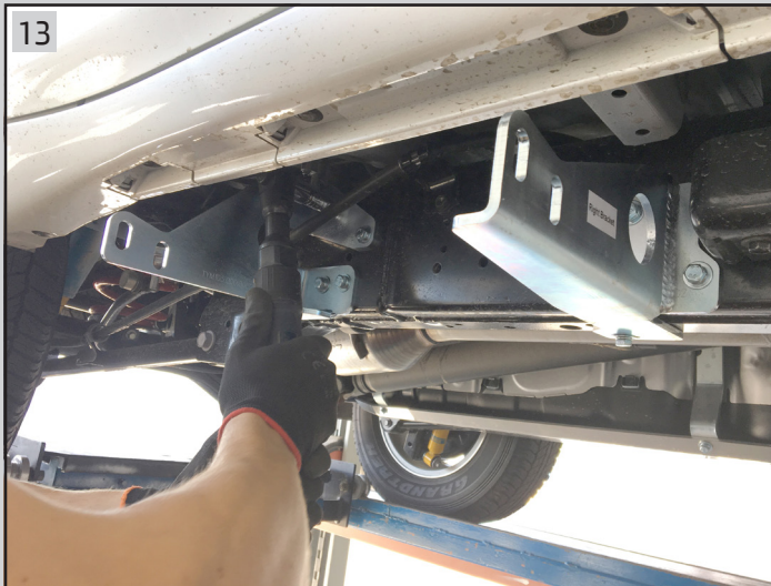
Tighten all 3 brackets bolts
